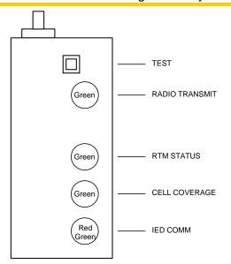
Press the Test button to test cellular signal strength
